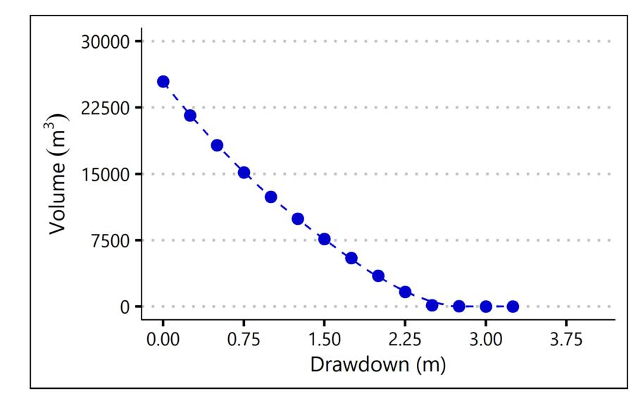
Water volumes are determined using detailed designs, as-builts, and/or volume tables when available. If design information is limited, then a bathymetric survey is used to measure pond volume. The decreasing relationship between volume at particular drawdown levels allows pesticide applicators to estimate volume quickly in the field immediately before treatment so as to achieve the desired concentration precisely.
